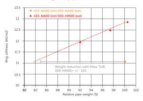
Amongst commercially available High Modulus PP materials, Eltex® TUB 350-HM00 delivers one of the lowest weight pipe that meets the normative requirements of EN1852 and EN13476.
