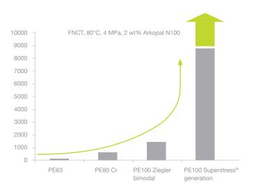
Slow Crack Growth Resistance of ELTEX® Superstress® resins exceed several years under FNCT (80°C, 4 MPa, 2 wt% Arkopal N100) exhibiting outstanding resistance against overall slow crack growth mechanism.
