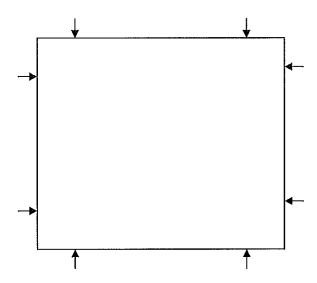
Three test plaques were obtained from random samples saved from each molding. Every shrinkage datum, length or width, was averaged from six readings (2 readings/each plaque x 3 test plaques)
