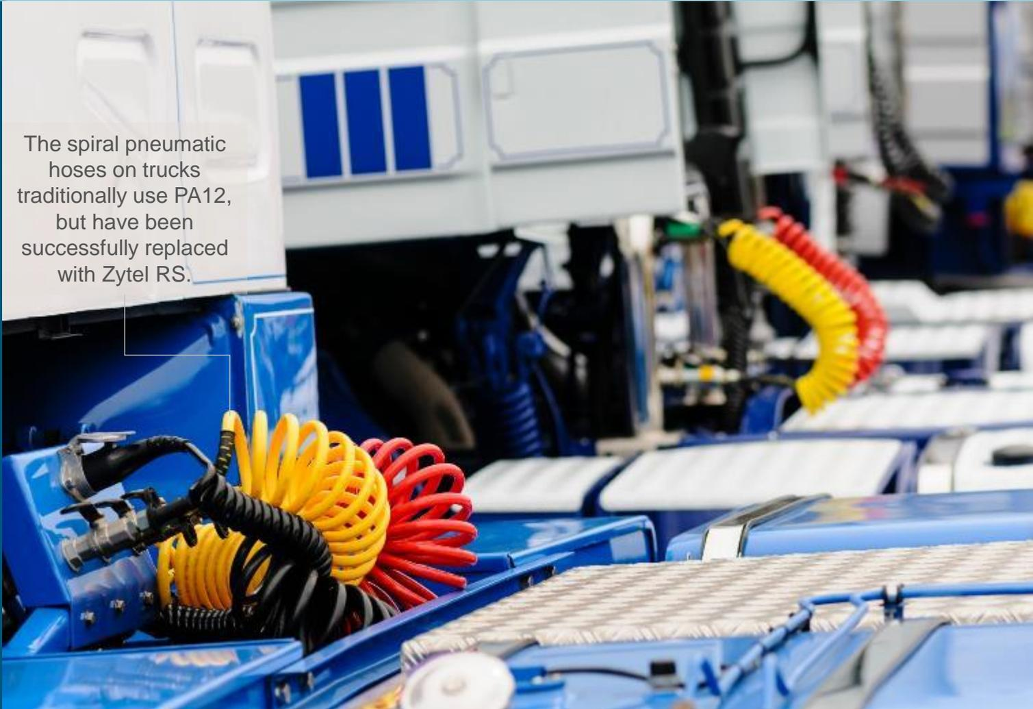
The spiral pneumatic hoses on trucks traditionally use PA12, but have been successfully replaced with Zytel RS.
