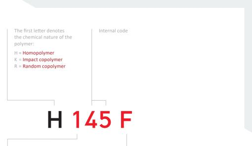
The **first digit** in three-digit numbers and the first two-digits in four-digit numbers indicate the melt flow rate (MFR) range in [g/10 min] at 230 °C and 2.16 kg
