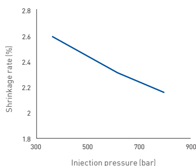
Fig 2-9. Shrinkage rate changes with injection pressures (F20-03, Melt temp. 200 °C, Specimen dia. 100 mm, t 2)
