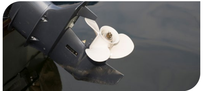
The stiffness and strength qualities of Rynite® are key factors in limiting blade deflection and preventing deformation in boat propellers.
