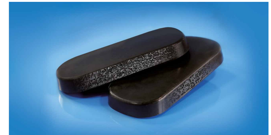
Figure 8: Foam structure with good and poor nucleation
