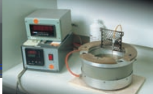
Fig. 15 Measuring shrinkage in a silicon oil bath.
