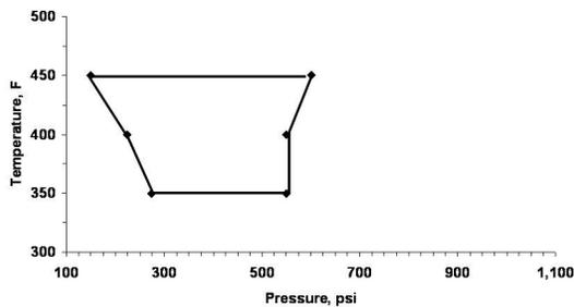
When selecting a flow for a molding setup, we recommend one with which parts can be molded at melt temperatures between 400 and 450°F at injection pressures between 1000 and 1500 psi. We also recommend selecting the lowest flow resin that will run under the above limits. Lower flow resins will have higher molecular weights and should produce molded parts with better toughness properties. Common problems resulting from use of resins with flows that are too high for a setup include:
