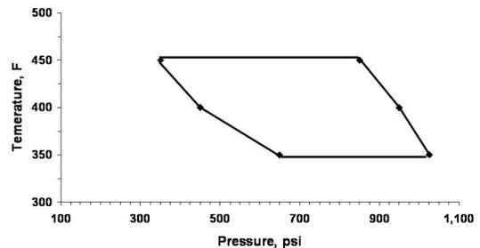
Figure 5: Molding area diagram for 5 MFR nucleated antistat
