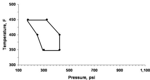
Figure 9: Molding area diagram for 35 MFR nucleated antistat
