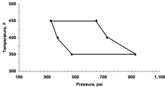
Figure 8: Molding area diagram for 35 MFR general purpose
