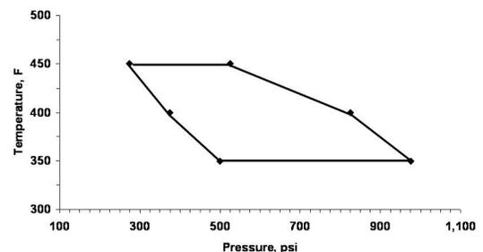
Figure 7: Molding area diagram for 12 MFR nucleated antistat
