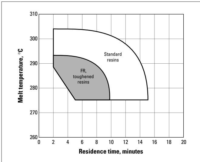
Fig. 3.4 Processing range: PET melt temperature vs. residence time
