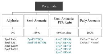
Based on semi-aromatic structure, Zytel\* HTN offers a balance of chemical, moisture and temperature resistance, plus outstanding processability.
