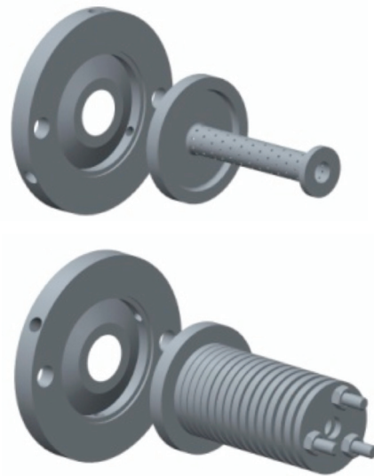
ANNULAR WATER RING & TUBULAR SIZING DIE WITH HOLES OR WITH PLATES
