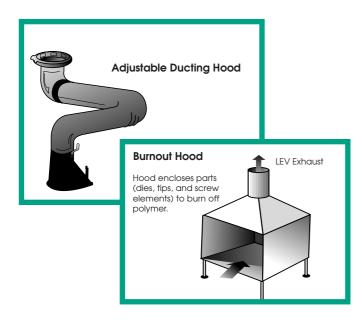
2. The hood should be shaped to enclose the source as far as is practical yet still allow access to the equipment for normal operation. The hood should be removable or connected to an adjustable duct that can be moved aside from extrusion or moulding equipment for maintenance or trouble-shooting. Adjustable ducting of this type is commercially available. Care should be taken to avoid kinking or excessive length of flexible tubing.
