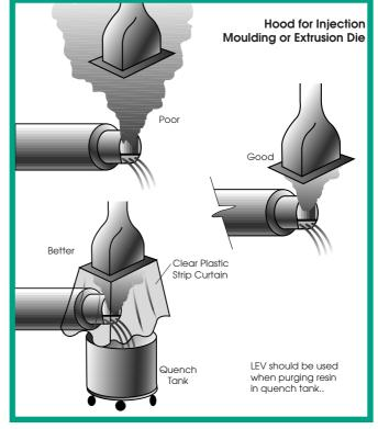
**5**. The capture effectiveness of a hood can be improved by using flanges (see Components of LEV System sketch). The flanges restrict airflow from behind and from the sides of the hood and maximize airflow from the front.
