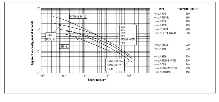
Figure 2. Apparent melt viscosity vs. temperature at a shear rate of 100  $\mbox{s}^{-1}$
