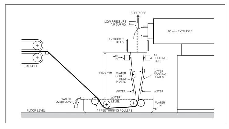
In practice, it has been found that due to the combination of the large diameter and thin wall section, flotation occurs after the extrudate leaves the sizing die. This can create a problem in maintaining a good vacuum seal.
