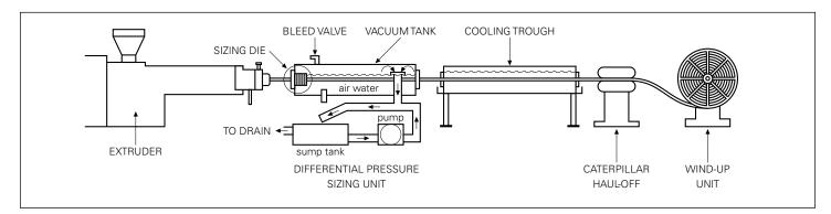
The fine adjustment to tube dimension is achieved, however, by adjustment to the vacuum applied to the vacuum bath.
