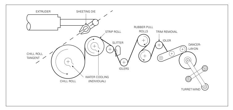
The processing conditions of melt temperature, quench temperature, air gap and extrusion rate all influence film properties, but quench temperature and air gap have the greatest effect. The following general statements indicate how each of these conditions affects film properties; the degree to which the property is affected depends on the grade of Hytrel<sup>®</sup> used:
