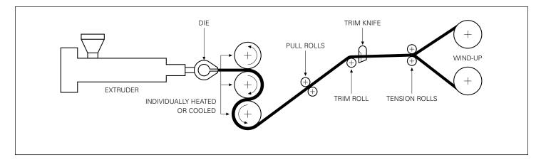
Roll temperatures should be individually controlled. Typical roll temperatures for Hytrel<sup>®</sup> sheeting extrusion are as follows:
