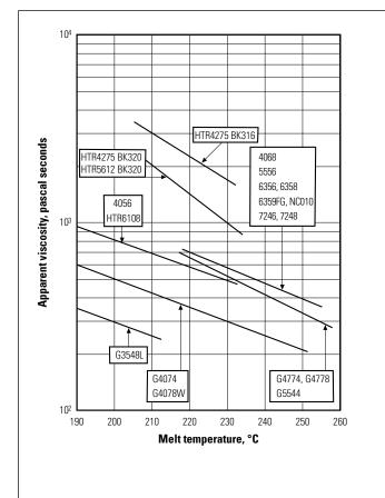
From **Figure 2** it can be seen that a significant change in melt viscosity can result from a relatively small change in melt temperature. The extrusion melt temperature can therefore be decreased (within limits) to provide greater melt strength for improved stability of the extrudate. It also means that good control of melt temperature is an important factor in successful extrusion of Hytrel<sup>®</sup> resins.
