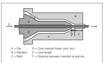
The clearance between the core to be covered and the bore of the "torpedo" or mandrel should be between 1% and 5% of the core diameter (depending on the material and regularity of the core surface).
