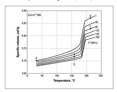
at the end of crystallization (point D), the part is solid and it can be ejected immediately; the molding shrinkage is the difference between the specific volumes at the crystallization temperature (point D) and at room temperature (point A).
