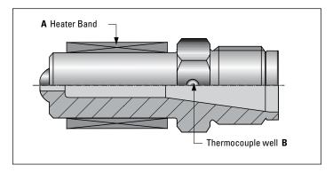
Screw decompression or "suck back" is frequently used to make control of drool easier with these open nozzles. This feature is available in most machines.
