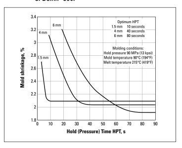
On the contrary, any increase of HPT above its optimum value would have no effect on mold shrinkage, because the part (and the gate) are already solidified.
