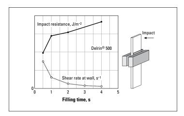
With non-optimum gate designs (conical, excessive gate length), shear in the gate may become an important limiting factor for part toughness.
