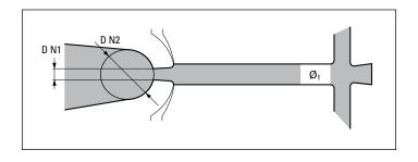
Figure 26. Example of a Design of a Nozzle Without Sprue Used with 2 Plate Molds. Remember that for Delrin® the Nozzle Temperature Should Not Exceed 190°C (374°F).
