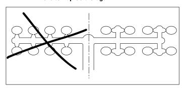
Figure 24. Example of "Spiral Effect" in a 32-Cavity Mold.
