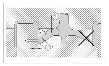
**Figure 19** shows details of a three plate gate design adequate for Delrin® (left), compared to a similar type of gate not recommended for crystalline materials. The design criteria illustrated above are also applicable to this kind of gate.
