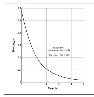
At 23°C (73°F) and 50% RH, Delrin® 100ST picks up 0.1% moisture in 4 hr; at 30°C (86°F) and 85% RH it will pick up 0.3% moisture in 2 hr. For this reason runners and sprues should be reground and reused as soon as possible.
