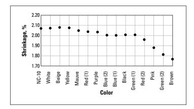
**Note:** This study has been carried out on standard bars and in typical molding conditions. The shrinkage values shown here should not be considered valid for all parts of different geometry and/or molded in different molding conditions.
