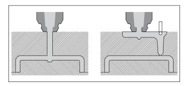
Figure 22. Balanced (Left) and Unbalanced (Right) Runner Systems in a 16-Cavity Mold
